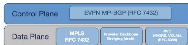
Figure 21-2: VXLAN Control Plane and Data-plane Definitions
